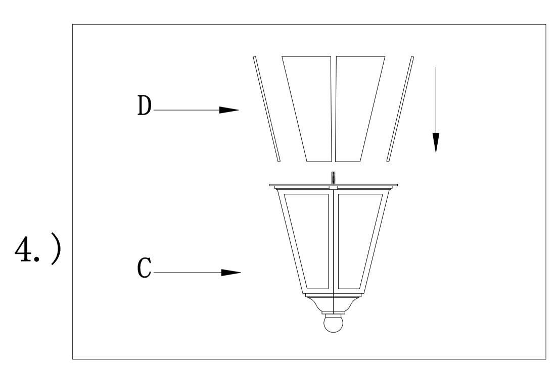
Step.4: Install the sheet glass(D) into the cage(C)
