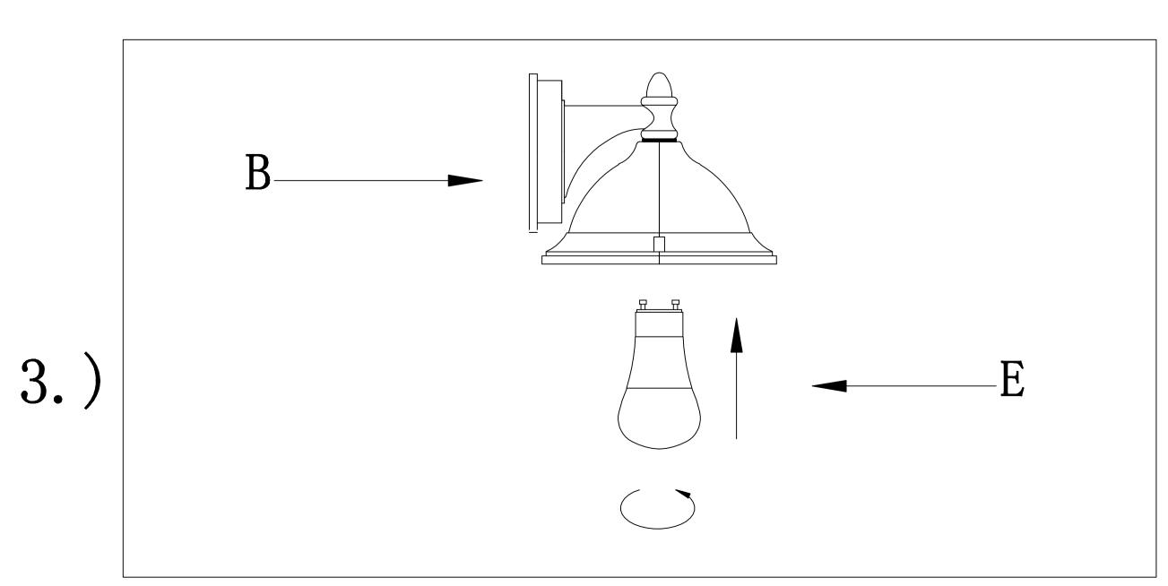
Step.3: Install GU24 LED bulb(E)
